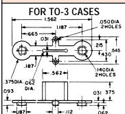
Barrier insulator, molded of type 6/6 natural colored nylon, functionally replaces up to six pieces of conventional insulation required with previous methods of mounting power transistors. Built-in barrier eliminates need for sleeving of connections.
